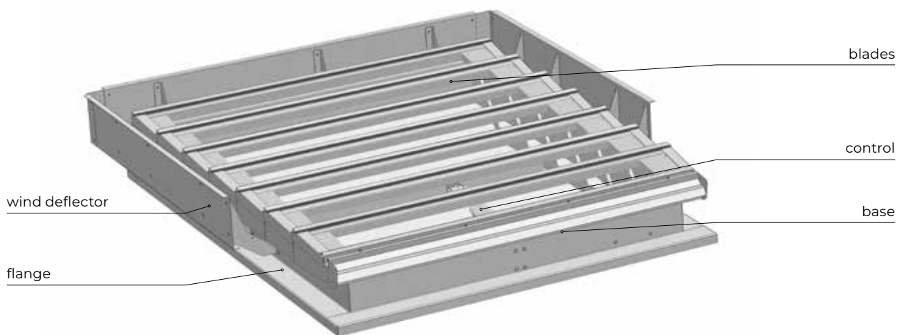
Fig. 1 Design of mcr LAM louvered smoke vent
